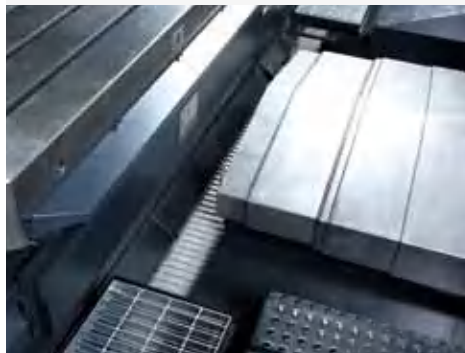
Built-in, hinge-type belt chip conveyor
